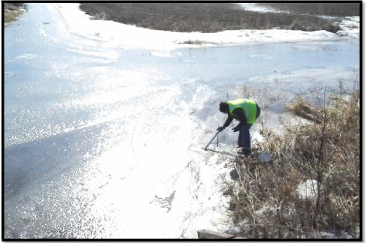
• Pennington County Soil and Water Conservation District staff helped collect manual stage measurements this spring until we were able to install water level loggers.
